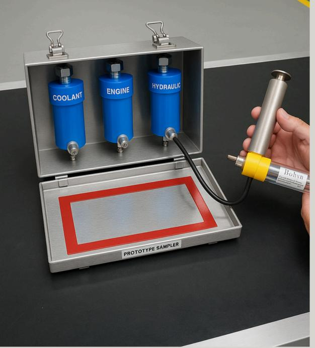
As the machine is shut down the spring loaded check valve shuts trapping approximately 120 ml of oil within the sampler. Once the machine is fully shut down and isolated the maintainer can lock onto the machine and take the sample from the sampler as required.
